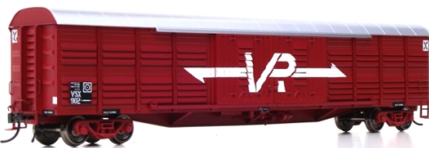
☐ Body V3 - Louvre Doors, No End Louvre Panel
